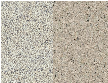
PT6 Block Paving Colour: Light Grey(60%), Light Cream (40%) 300x200mm, staggered bond Textured concrete block
